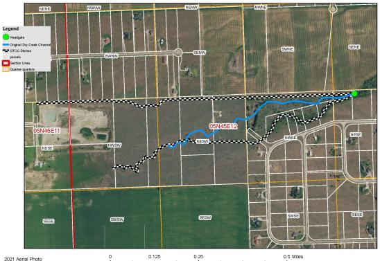
For this year, the Company only intends to engage in vegetation removal on the south ditch depicted on the map up to the headgate (depicted with a green dot), and then remove vegetation on the north ditch downstream of the headgate. The Company does not intend to do other vegetation removal for other parts of its delivery system associated with Dry Creek this year, but may in the future as necessary.
